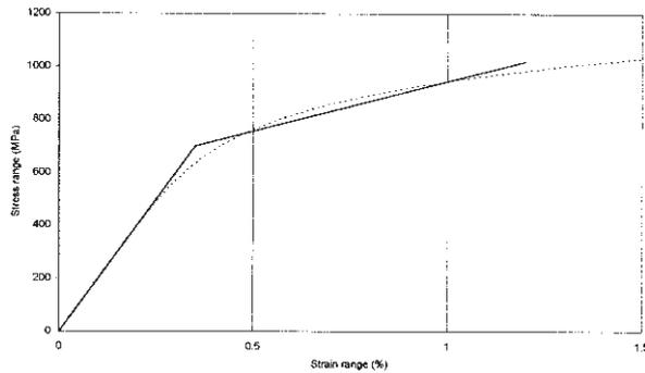
Figure C4 Construction of bi-linear model (solid line) from CSS data (dotted line).
