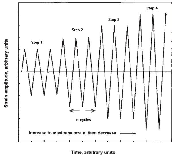
Figure 3 Typical multiple-step test (schematic).
