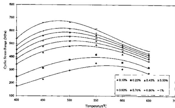
**Figure D1** Cyclic stress ranges as a function of temperature.
