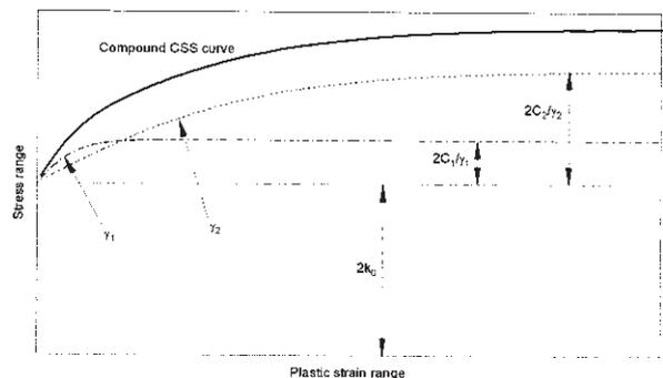
Figure 9 Illustration of the constitutive parameters on the shape of the CSS curve for a Chaboche type equation with two kinematic hardening variables.
