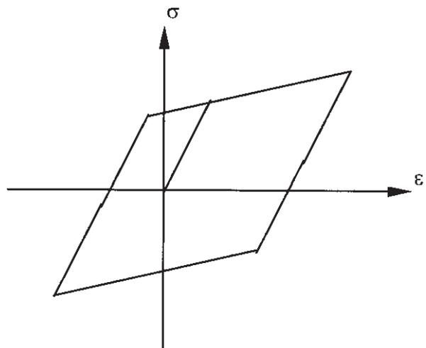
Figure C3 Schematic representation of bi-linear kinematic hardening.
