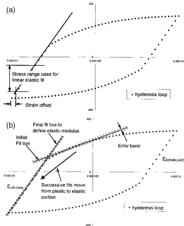
Figure 7 Methods for determining elastic modulus.
