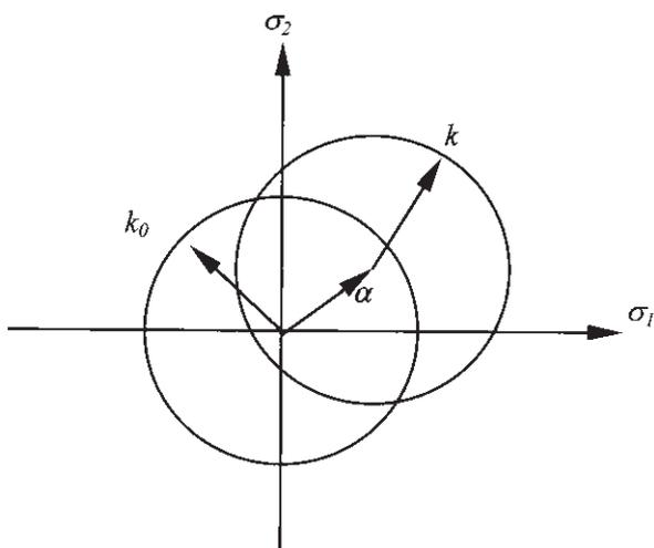
Figure C2 Schematic representation of kinematic hardening.
