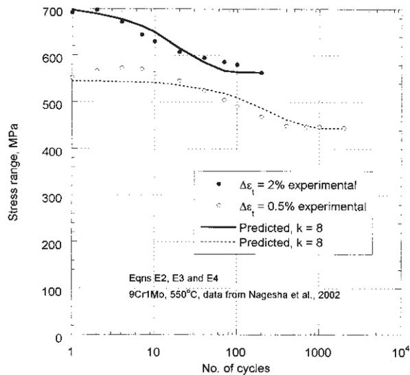
Figure E1 Prediction of cyclic softening in modified 9Cr1Mo steel at 550°C.
