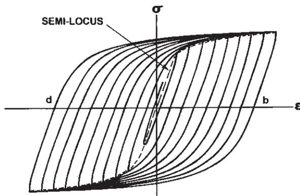
Figure 2 Typical incremental-step test (schematic).
