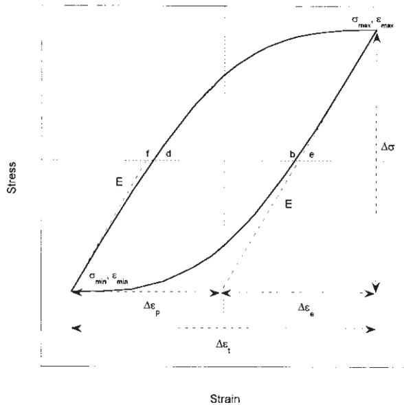
Figure 1 Terms used to characterise cyclic stress strain loop.
