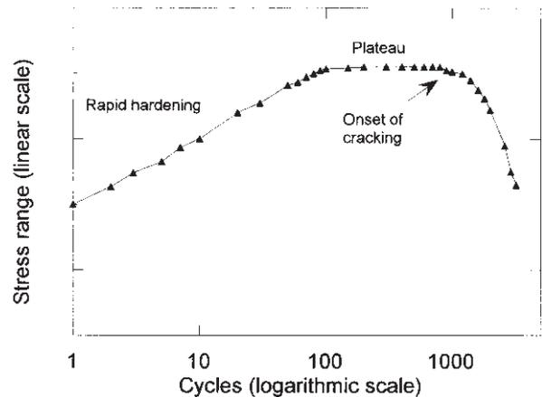
Figure 4 Variation of stress with time for cyclic hardening material.
