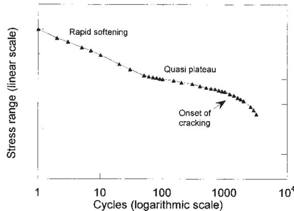
Figure 5 Variation of stress with time for cyclic softening material.
