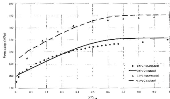
**Figure D3** Observed and calculated stress ranges as a function of cycle number for Type 304 steel.
