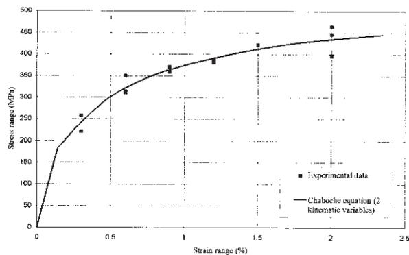
**Figure D4** Cyclic stress-strain curve for Type 304 steel (data points taken from Table D3).
