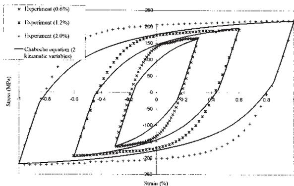
Figure D5 Comparison of experimental and predicted stabilised hysteresis loops for Type 304 steel.
