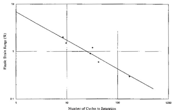
**Figure D2** Relationship between number of cycles to reach saturation,  $N_{sat}$ , and plastic strain range.
