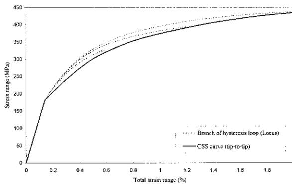
Figure D6 Comparison of CSS curve and individual hysteresis loops to demonstrate the 'non Masing' nature of the Chaboche model.
