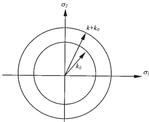
Figure C1 Schematic representation of isotropic hardening.
